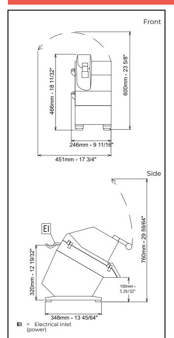
Electric 220-240 V/1N ph/50 Hz Supply voltage: Electrical power, max: 0.37 kW 0.37 kW **Total Watts:** Capacity: Performance (up to): 400 kg/hour Key Information: External dimensions, Width: 246 mm External dimensions, 557 mm Depth: External dimensions, Height: 466 mm **Shipping weight:** 21 kg
